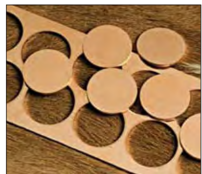
Rand Refinery has manufactured over 55 million blanks for minting into Krugerrands.
