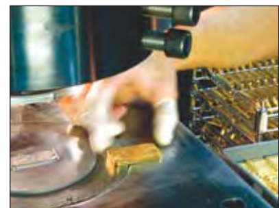
Manufacturing minted bars at PAMP (Switzerland).
