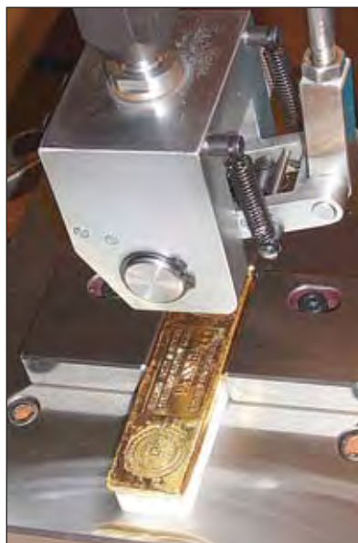
Hong Kong Good Delivery 5 tael bars (6.01685 oz) are stamped by The Chinese Gold & Silver Exchange Society.
