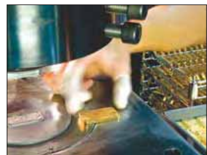
Manufacturing minted bars at PAMP (Switzerland).
