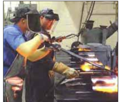
Manufacturing London Good Delivery 400 oz bars at Johnson Matthey (USA).
