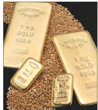
Kilobars are manufactured to a fineness of 995, 999 or 999.9 for the international market.
