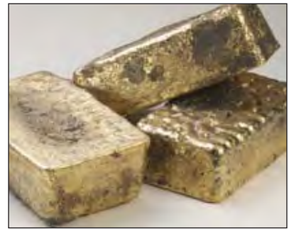
Low purity doré bars supplied by mining companies for refining into tradable bars.
