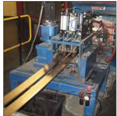
These long, flat bars, after rolling, will be cut with a die to produce blanks for minted bars.
