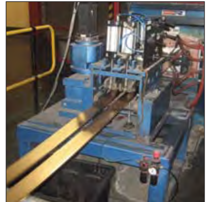
A continuous casting machine producing flat cast bars from melted gold.
