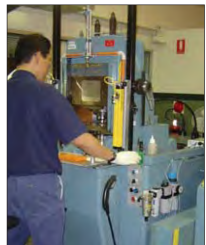
Striking the blanks between dies in a minting press.
