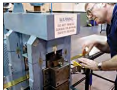
Rolling flat cast bars to the required thickness.
