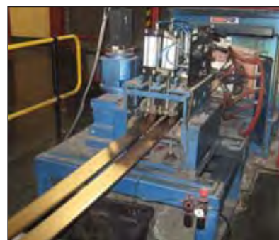
A continuous casting machine producing flat cast bars.
