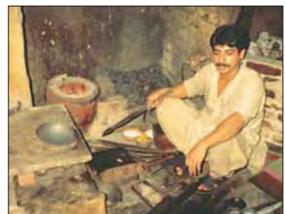
A "backyard refiner" in Pakistan manufacturing small tezabi bars.
