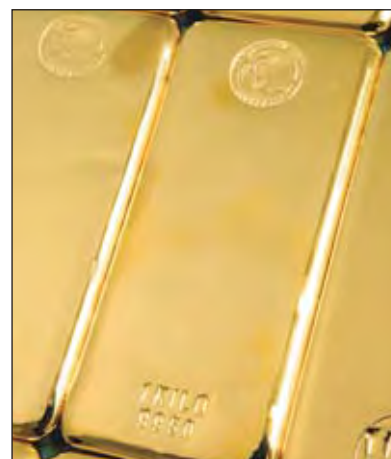
Kilobars are manufactured for the international market to a fineness of 995 or 999.9.
