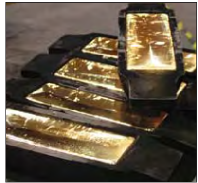
400 oz bars cooling in their bar moulds.
