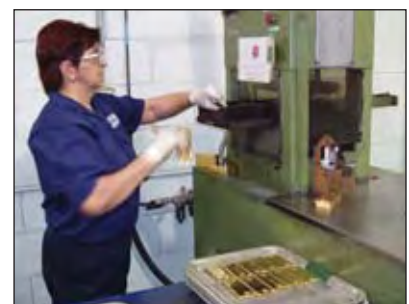
Applying official stamps and other markings to small cast bars.
