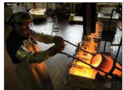
Pouring melted gold into a 400 oz bar mould.
