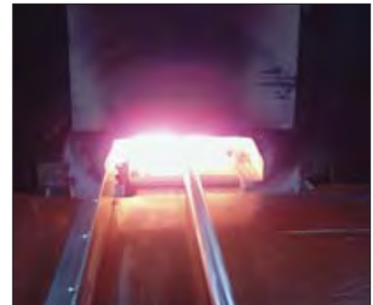
Pushing a group of bar moulds into an induction furnace.
