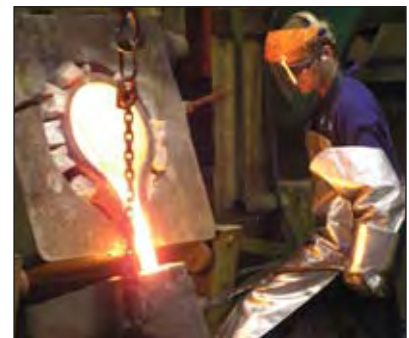
Pouring melted gold into a transfer crucible.
